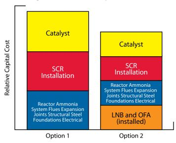
Combinations of low  $NO_x$  burners (LNB), overfire air ports (OEA) and selective catalytic reduction (SCR) equipment provide a very flexible system of  $NO_x$  control alternatives. As the graph shows, optimizing the entire combustion system will dramatically reduce the size and capital cost of the SCR system. SCR operating costs are also significantly reduced via this total design approach.
