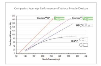
Compares peak impact pressure (PIP) of the Gemini sootblower nozzle and the Gemini low pressure (LP) sootblower nozzle, to previous Diamond Power high performance nozzles. The result is better cleaning at a wide-range of supply pressures.
