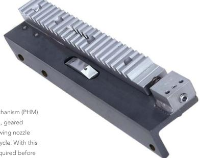
The Diamond Power® progressive helix mechanism (PHM) from Babcock & Wilcox (B&W) is a precision, geared indexing mechanism that shifts the sootblowing nozzle starting position by a known amount each cycle. With this device, hundreds of operating cycles are required before the nozzle repeats the same cleaning path. This allows for more complete cleaning coverage and significantly reduces tube damage due to erosion.
