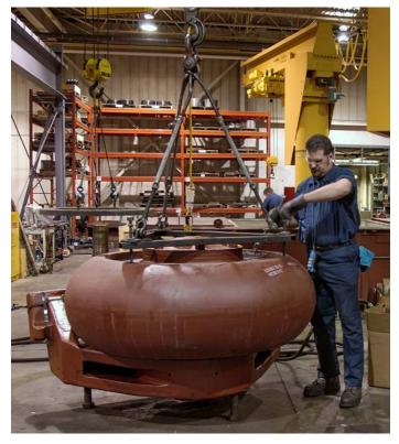
During B&W's rebuilding process, each part of the roll wheel assembly is inspected to OEM requirements to ensure product quality and integrity.
