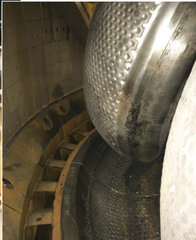
Xwin material technology from Magotteaux combines the extreme high hardness of ceramic with the mechanical properties of high chromium metal for maximum wear resistance and wear life.
