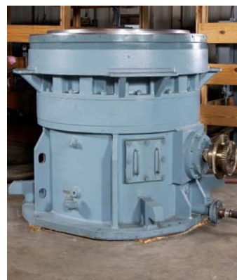
The planetary geardrive is the standard offering for most pulverizer installations.
