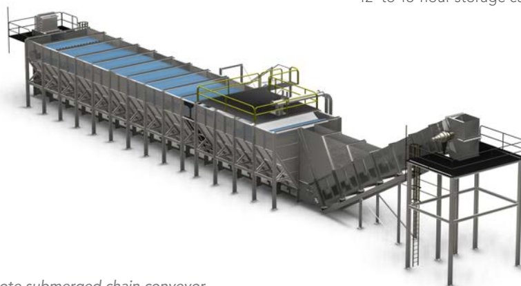
Remote submerged chain conveyor
