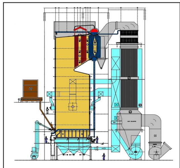
**Fig. 1** Typical economizer and tubular air heater arrangement.
