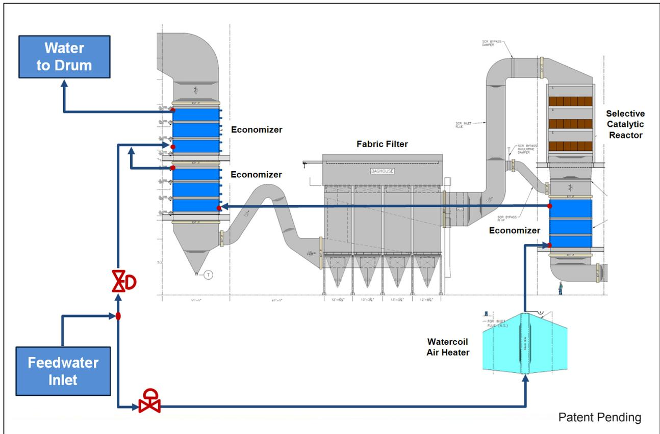
Fig. 2 Air quality control system temperature control.
