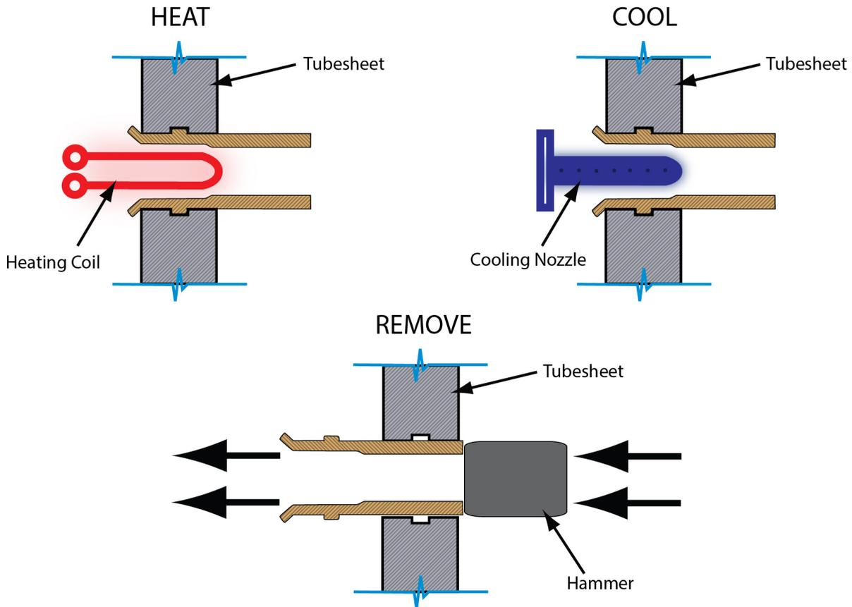
Both methods eliminate the need for conventional carbon arc or acetylene splitting of the tube stubs as well as the potential damage to the tube seats and subsequent repair requirements.
