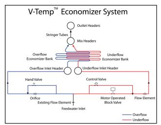
Fig. 1 V-Temp economizer system schematic.
