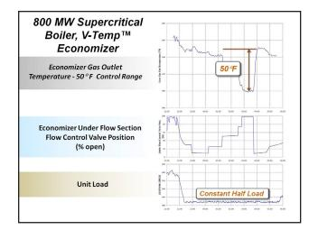
Fig. 11 V-Temp economizer test control range.
