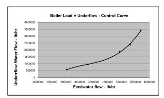
Fig. 10 Control curve – boiler load vs underflow rate.
