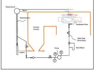
Fig. 13 Furnace/downcomer recirculation system.
