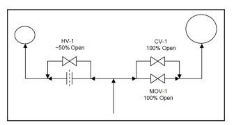
**Fig. 8** Valve positions – start-up to minimum load required for SCR operation.
