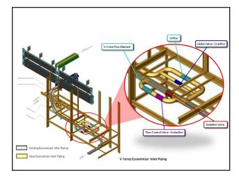
Fig. 3 Expanded view of V-Temp system.
