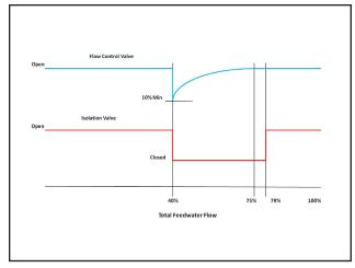
Fig. 9 Valve positions across the load range.
