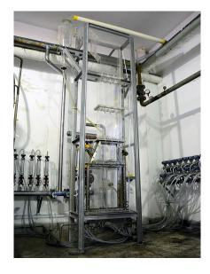
**Figure 5**. Cold Flow Model Constructed of Plexiglas<sup>®</sup>, <sup>1</sup>/<sub>4</sub> Scale of Hot Pilot Plant, Used to Validate System Hydrodynamics
