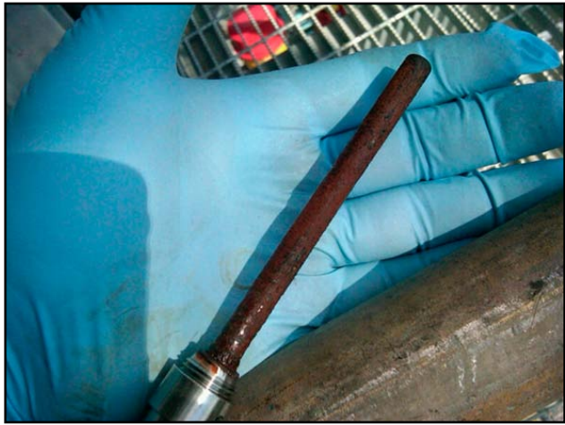
Figs. 3a and 3b ER probe (left) and WL coupons (right).
