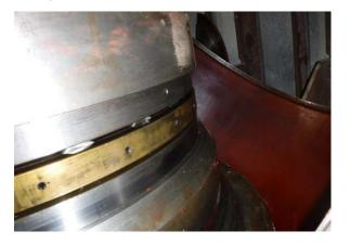
Owners should adopt a periodic inspection of the air heater bearings during planned outages. Access to conduct a detailed inspection, after partial disassembly of the bearing housings is limited, so only parts of the bearings are viewable. If owners have concern, replace the bearings and inspect the old bearings in a shop or laboratory to see if they are adequate as spares. The continually loaded thrust bearing is expected to be the bearing that would initially fail.
