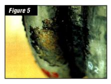
has occurred (Figure 5), requires that all areas of exposed carbon steel be weld-overlayed with Type 309L stainless steel.
