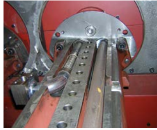
Water-cooled DynaGrate with cooling integrated in shaft.
