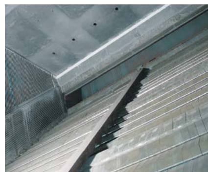
The unique design and movement of the DynaGrate combustion grate minimizes maintenance and optimizes fuel burnout.
