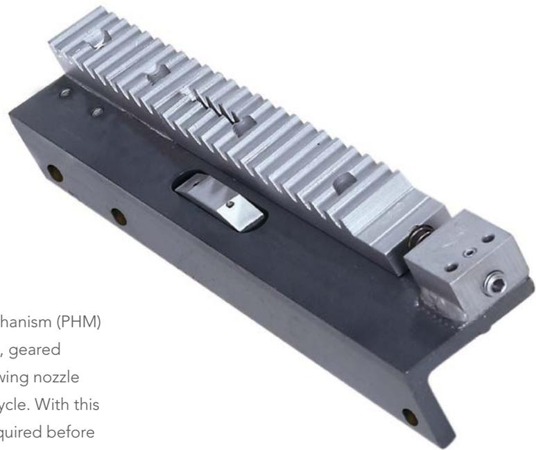
The Diamond Power® progressive helix mechanism (PHM) from Babcock & Wilcox (B&W) is a precision, geared indexing mechanism that shifts the sootblowing nozzle starting position by a known amount each cycle. With this device, hundreds of operating cycles are required before the nozzle repeats the same cleaning path. This allows for more complete cleaning coverage and significantly reduces tube damage due to erosion.
