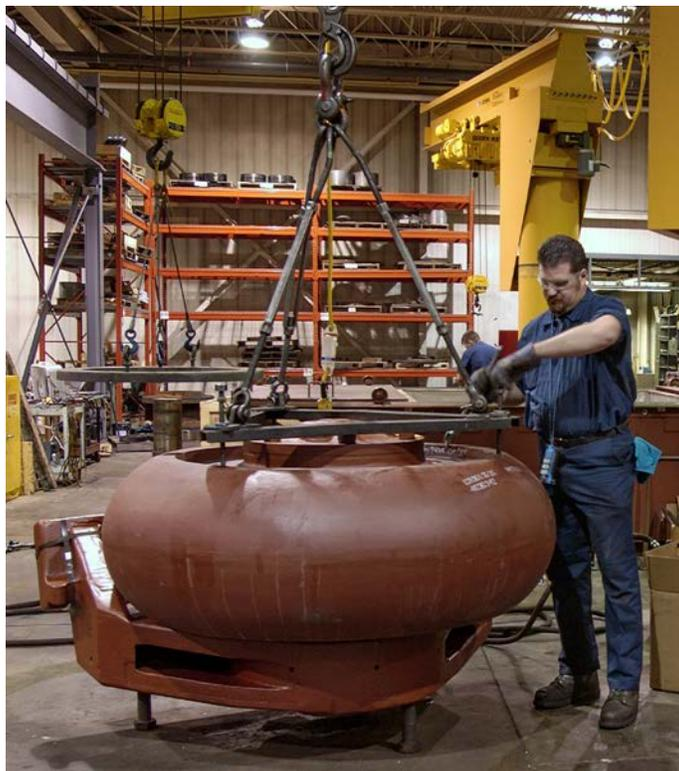
*During B&W's rebuilding process, each part of the roll wheel assembly is inspected to OEM requirements to ensure product quality and integrity.*
