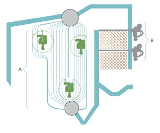
The elevation at left shows a typical Diamond Power G9B sootblower system. The arrangement shows (A) three convection-section G9B blowers and (B) two of the four G9B installed in the economizer at the rear of the boiler.
