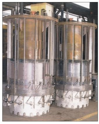
Like all B&W combustion equipment, the parts exposed to the radiant furnace heat are constructed of high temperature alloy material (bottom of photo) ensuring long life and durability.
