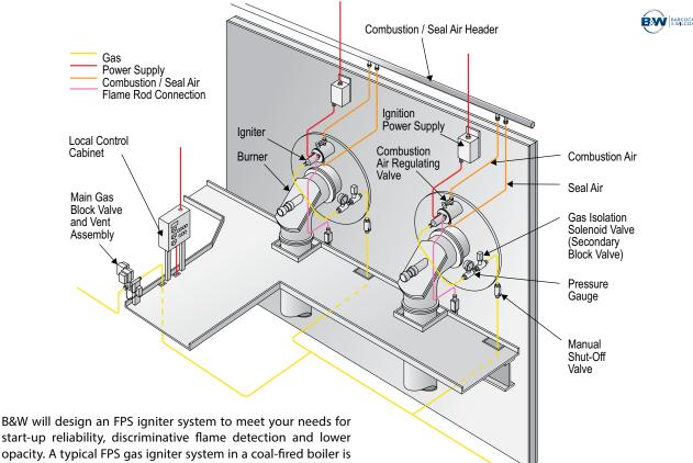
start-up reliability, discriminative flame detection and lower opacity. A typical FPS gas igniter system in a coal-fired boiler is illustrated above with in-line valving.
