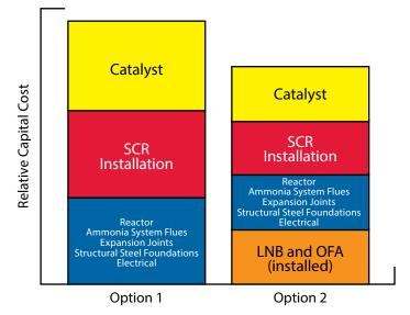
Combinations of low NO<sub>x</sub> burners (LNB), overfire air ports (OFA) and selective catalytic reduction (SCR) equipment provide a very flexible system of NO<sub>x</sub> control alternatives. As the graph shows, optimizing the entire combustion system will dramatically reduce the size and capital cost of the SCR system. SCR operating costs are also significantly reduced via this total design approach.
