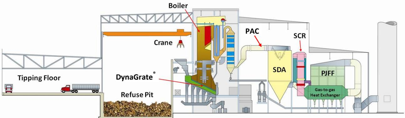
**Fig. 5** Side view of PBREF No. 2 looking west showing one of three process lines. (Not shown: turbine generator behind and metals recovery/ash management in the foreground)
