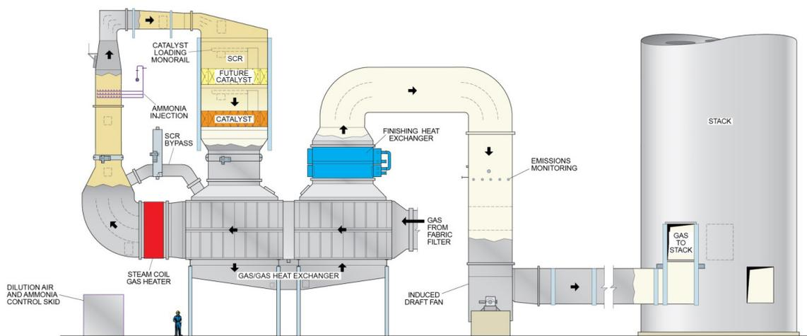
**Fig. 12** SCR reheat and heat recovery system.
