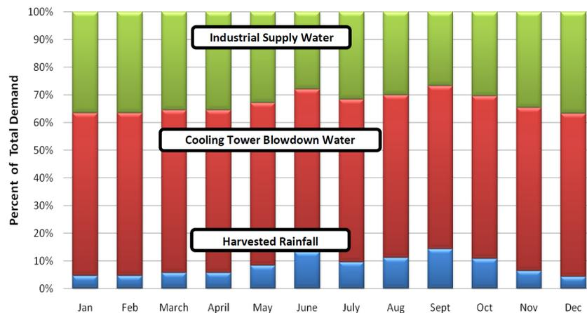
**Fig. 6** Nominal water supply sources for PBREF No. 2.
