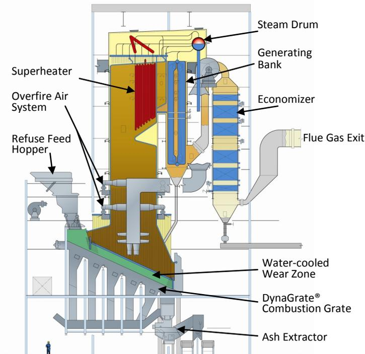
**Fig. 7** B&W Stirling® mass burn power boiler schematic.
