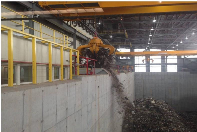
**Fig 10** Automated refuse crane technology.
