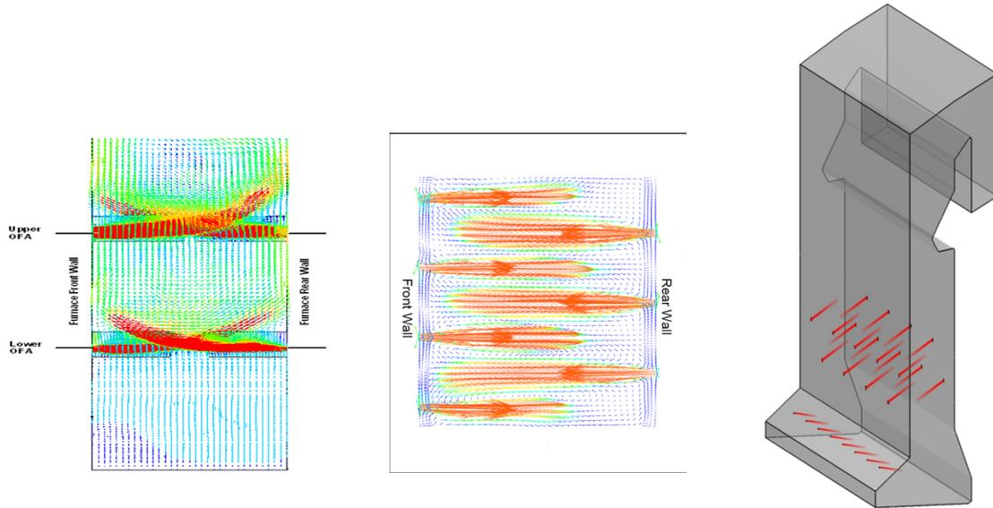
**Fig. 9** Combustion modeling for PrecisionJet® air system.
