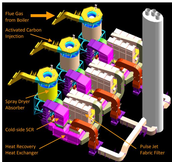
**Fig. 11** Post-combustion emissions control technology.
