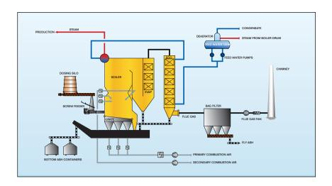
The plant is equipped with a water-cooled vibrating grate. The different types of fuel receive preliminary treatment in order to divide the fuel into smaller particles and to mix the wet and dry material.
