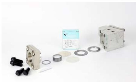
Gasket kit with gauge glass — 1050 psi; Ruby mica – retorqueing required 24 hours after installation
