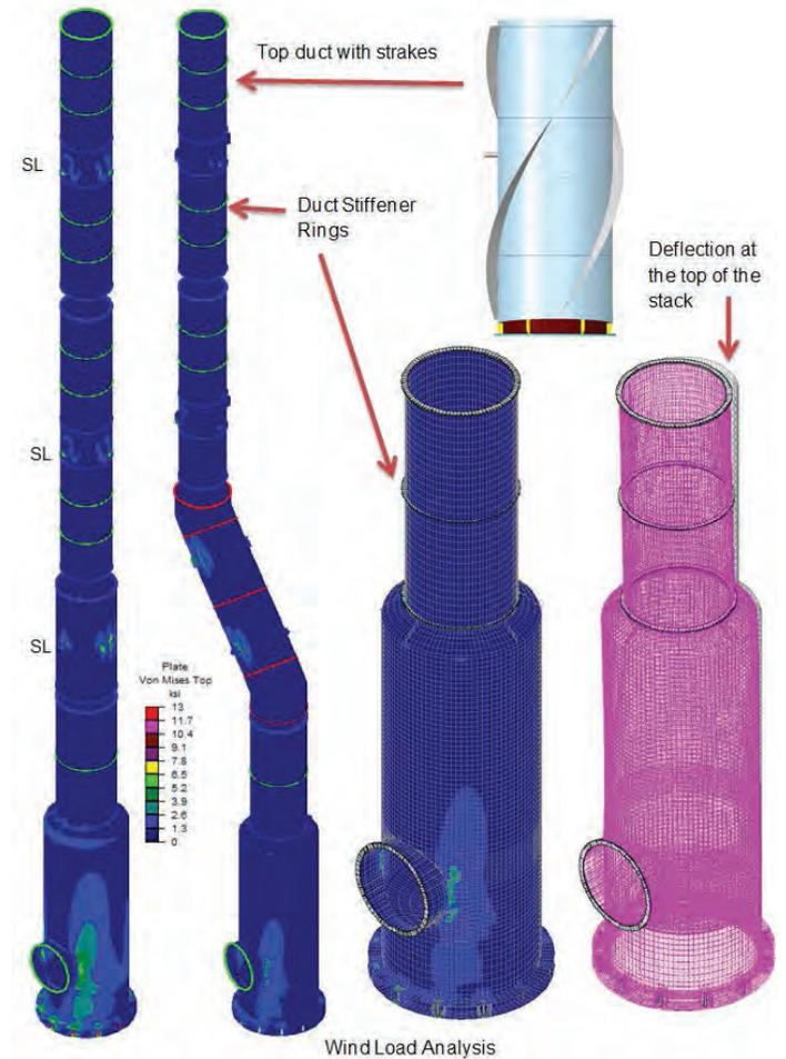
Fig. 5. Schematic view of the wind load analysis results for the straight and partially slanted vertical stack systems. Note the top duct with strakes per ASME STS-1 recommendations.
