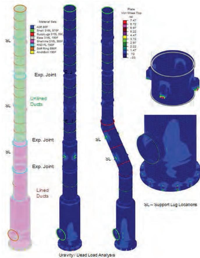
Fig. 4. Schematic view of the stack components and dead load analysis results for straight and partially slanted vertical stack systems.
