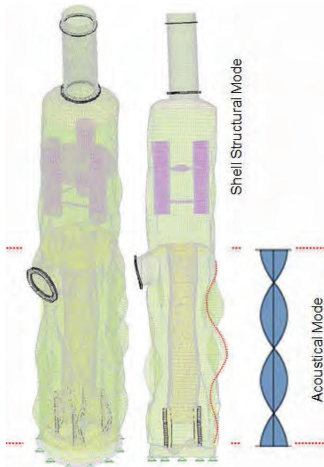
Fig. 8. Silencer structural resonant frequencies close to the dominant firing frequencies and acoustic modal frequencies.
