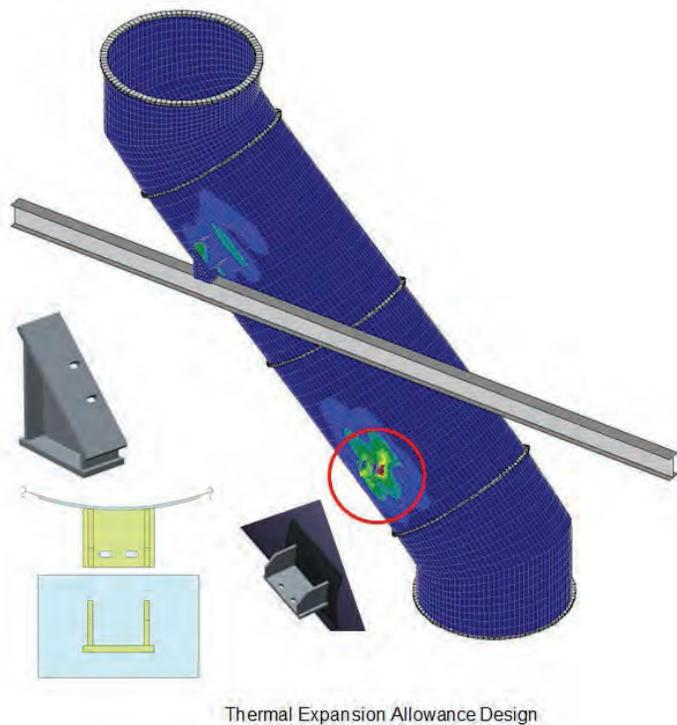
Fig. 7. Schematic view of the slanted duct support lug configurations. Note slotted bolt holes on the support lug and welded “I” beam seat to allow thermal expansion at the support locations.
