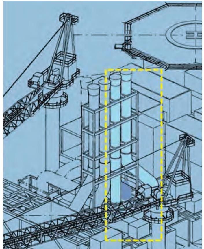
Fig. 2. Isometric view of the analyzed vertical and partially slanted vertical exhaust systems.
