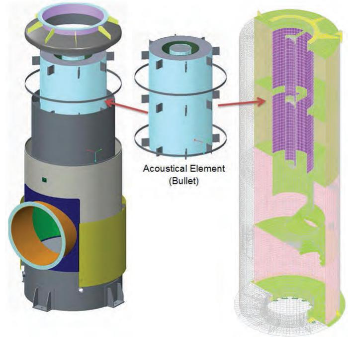
Fig. 3. Isometric view of the typical silencer including the acoustical element (bullet) on the left and middle, and FE modeling example to the right.
