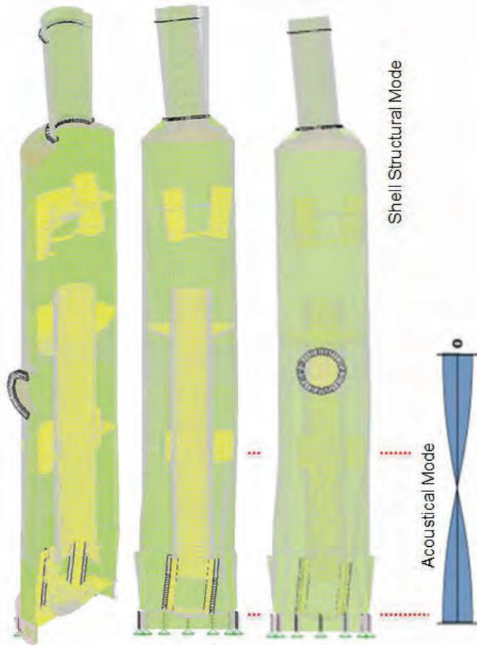
Fig. 9. Improved silencer design including acoustic and structural resonant modes/frequencies not aligned with the dominant firing frequencies.
