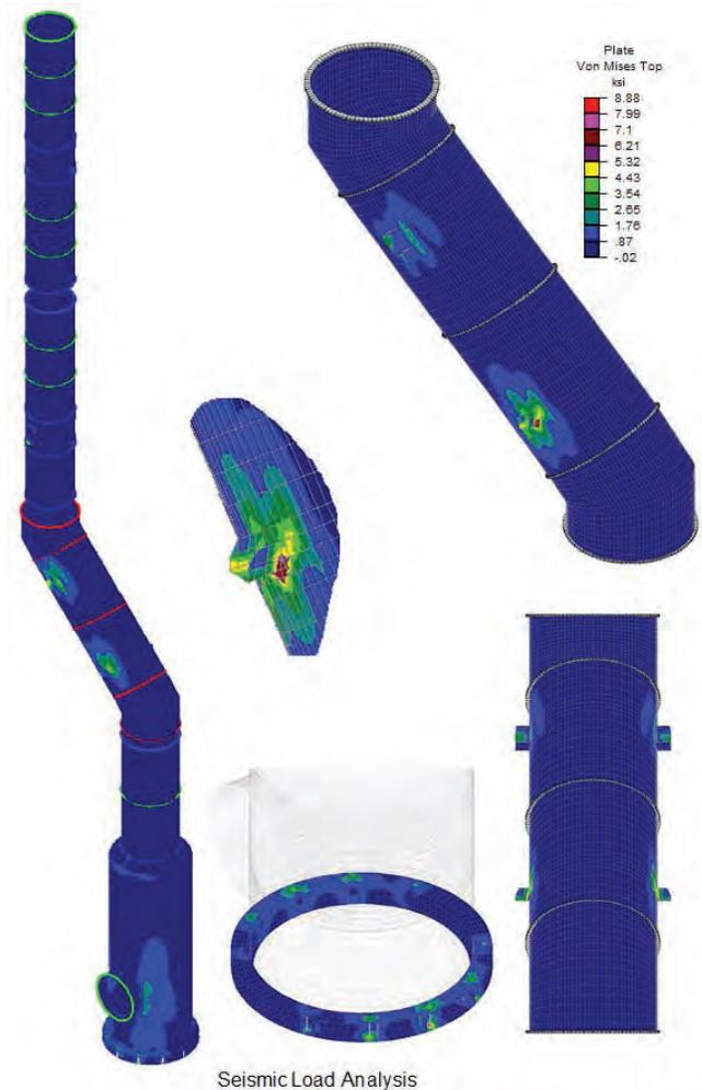
Fig. 6. Schematic view of the seismic analysis results for partially slanted vertical stack system. Note stress concentration at the shell support lugs and base ring anchor bolts.
