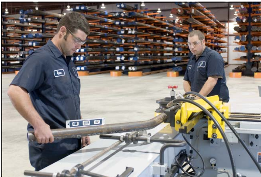
B&W's expanded tube stocking facility also includes bending capabilities for exact radius bends as specified by the customer.
