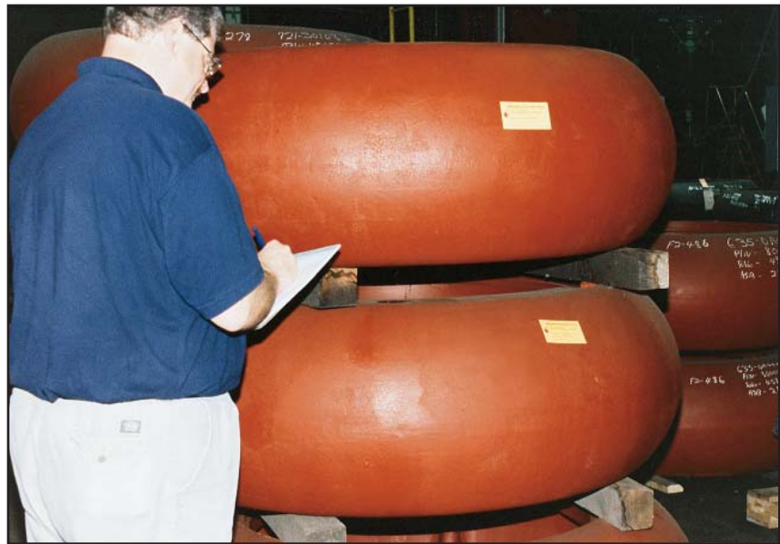
Designed for extended service life, the Wearesistor asymmetric tire includes additional premium wear material in the high wear areas.
