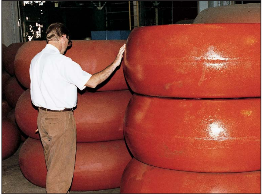
The top two tires pictured in the foreground are B&W PGG's Wearesistor LP tires. The low profile geometry can be seen when compared to the other standard tires in the picture. When combined with our low profile segments, this exclusive design significantly extends the operating life of both components.
