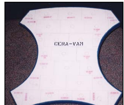
Pulverizer turret panels with Cera-VAM ceramic lining provide added protection against wear at the top of the pulverizer turret.
