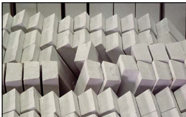
Typical Cera-VAM bricks for lining pipe are about 1 in. thick, 2 in. wide, and 9 in. long (25.4 mm x 50.8 mm x 228.6 mm) and weigh about 22 oz (623.8 g) each. Specially designed 6 to 9 degree angled edges create a keystone effect to help lock bricks in place.
