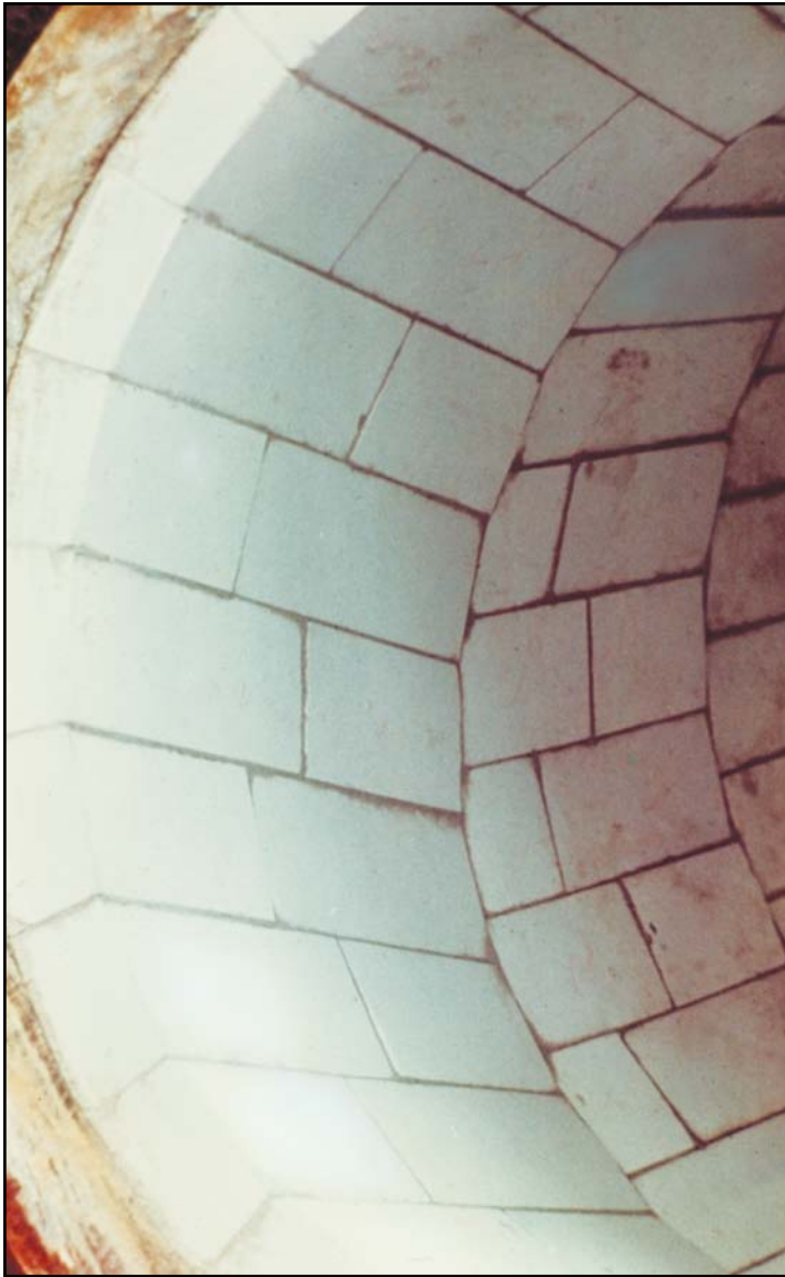
Cera-VAM bricks are pre-formed to follow the bends of burner line elbows.
