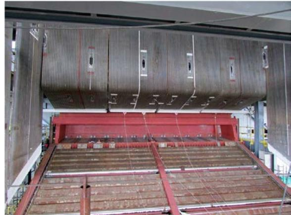
A view inside the furnace shows the fuel ram feeder, B&W Vølund DynaGrate® wave moving grate combustion system, and weld overlay for lower furnace tube corrosion protection.
