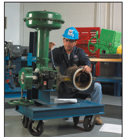
Skilled technicians perform valve actuator overhaul and refurbishment.
