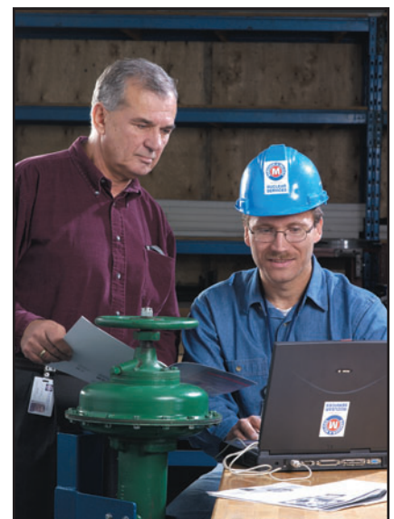
Performing diagnostic testing of air operated valve to set-up the valve performance criteria and meet system requirements.
