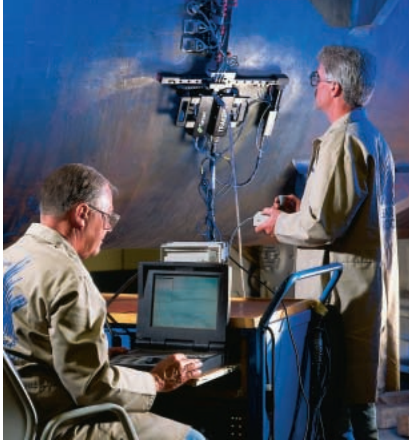
The Tomoscan® system's robotic scanner easily makes simultaneous, multiple scans, stores your data, and gives you complete coverage of a circumferential weld seam.
