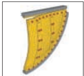
Elastic-plastic Large Deflection Failure Analysis of a Divider Plate under LOCA loading
