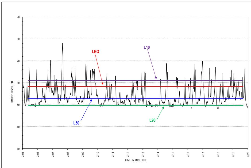
Figure 1 – Environmental Sound Level Vs. Time Near a Road
