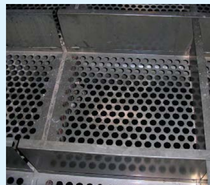
B&W's absorption tray provides uniform gas flow and maximizes SO 2 removal. This photo shows a tray after two years of continuous service.
