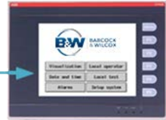
The local control panel consists of a PLC with touchscreen operator interface to control the hose cart and water supply pump.
