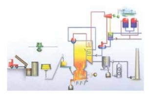
Using Vølund™ technology, B&W designed the boiler for firing a wide range of biofuels, which will consist mainly of forest wood chips with up to 55% moisture, sawdust, chipped clean wood from industry, and wood pellets.
